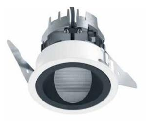
Specialists for high rooms Recessed luminaires for high rooms require high luminous flux and precise optics. A lens system consisting of collimator and Spherolit lens transforms Quintessence double focus downlights into specialists for such applications. The innovative lighting technology of the wallwashers enables particularly close distances to the wall. The black anti-glare cone achieves high visual comfort and a discreet appearance.
